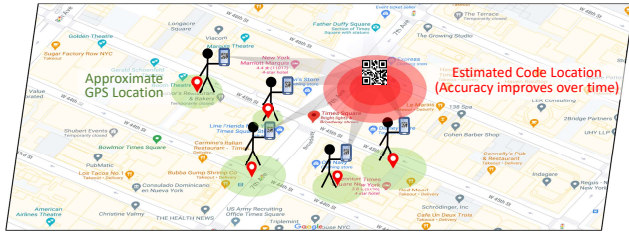
Figure 4: Code localization. Approximate locations of users who successfully scanned a full code are used to estimate the location of the code. The estimate becomes more and more accurate as more users scan the code.
