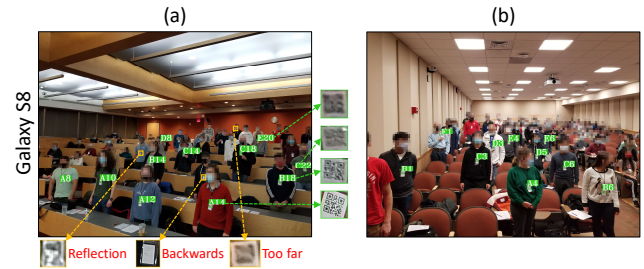
Figure 13: Case study: attendance tracking with context-guided pruning. Correctly decoded codes are shown in green labeled with seat numbers. Three failure modes are highlighted in yellow. Most codes within 7m can be decoded, which suggests QfaR can be a potential solution to automated attendance systems.
